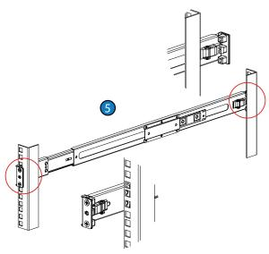
Mount the slide rails to the frame of the rack. Attach the ends to the frame and press the bracket to fix the rail onto the frame.
