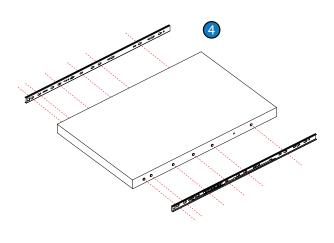
Mount the inner rails on the server chassis.
