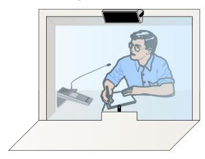
The client-side loudspeaker must be mounted at least 50 cm (19.7 in) away from the client-side microphone and, if possible, should not face the microphone directly because this leads to an echo of the operator's voice on the client side. It is recommended to choose one of the following mounting versions:
