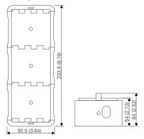
For mounting of an Outdoor series Intercom station in the flush mount box XDX FBS, the gypsum/panel mount kit XDX FB is required.
